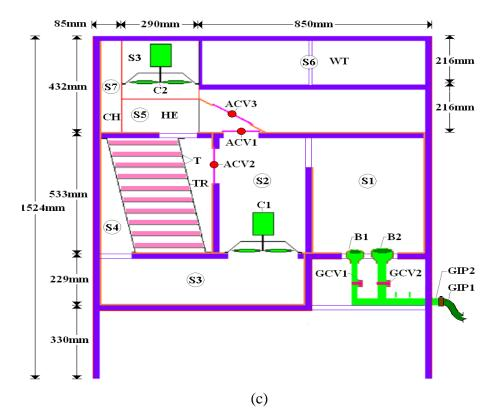
Fig. 4 (a) Graphical view and (b) external view of the proto-type and (c) view showing different components of the batch type tea dryer
