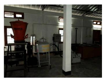
Fig. 5 Commercial biomass gasification unit for generation of producer gas
