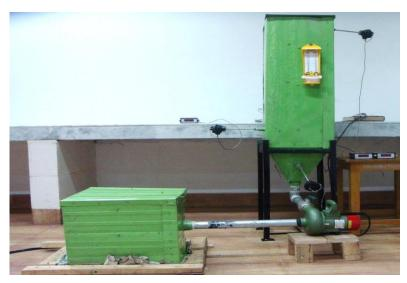
Fig. 7 laboratory setup of two stage fluidized bed dryer.
