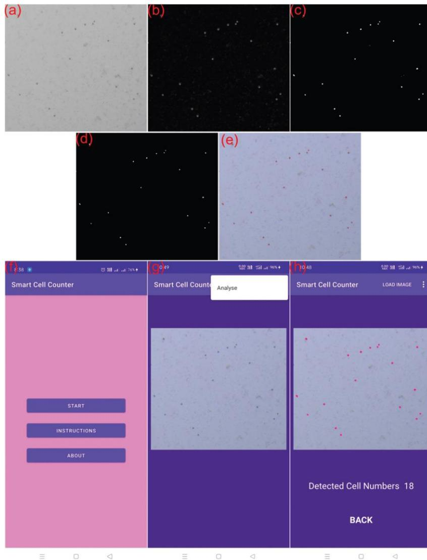
Fig.5 Development of the cell recognition and counting algorithm and the interface of the android application. (a) BF image of cells in a single FOV; (b) implementation of the Sobel operator to recognize the cell boundaries; (c) threshold image; (d) recognized cells after the removal of noisy artifacts; (e) cell number estimation using contour detection algorithm; (f ) initial interface of the android app; (g) BF image read-in; (h) output results.
