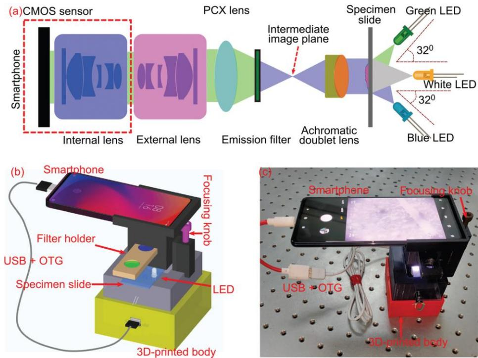
Fig.2 Design of the proposed Bright Field and fluorescence microscopy device. (a) Optical layout diagram of the system; (b) 3D design of the system; (c) fully assembled device
