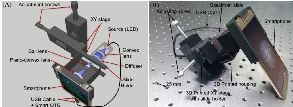
**Figure 2:** Smartphone based microscope: (A) the optical layout, (B) the 3D printed prototype installed on an android smartphone device.
