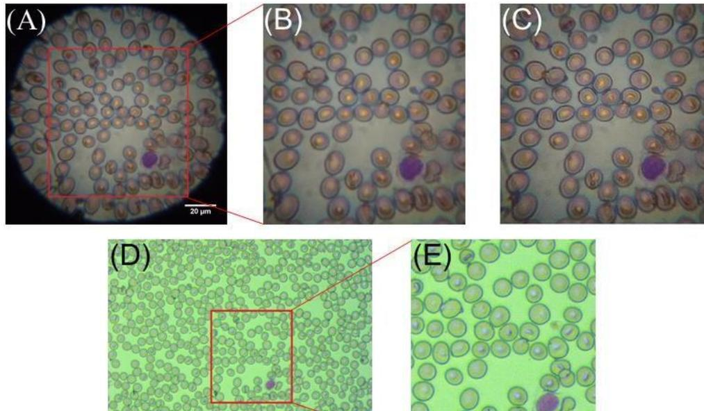
**Figure 5:** Processed smartphone microscope image of thin blood smear. (A) Smartphone microscope image, (B) corresponding image of a cropped region, (C) corresponding processed image of the cropped region (D) a 40X/0.65 NA traditional microscope image of the blood sample and (E) zoomed version of the same region of interest (ROI) of the traditional microscope. Scale bars are 20  $\mu\text{m}$ .
