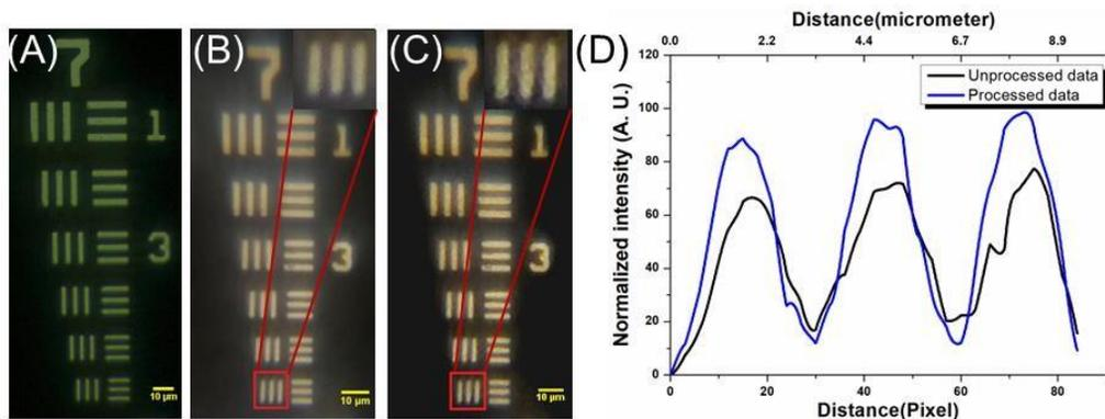
**Figure 4:** Images of USAF Resolution test target (A) obtained from standard optical microscope (Carl Zeiss's Primo Star), (B) with the designed smartphone based optical microscope, (C) its corresponding processed image and (D) intensity profile of the selected region. Scale bars are  $10 \mu\text{m}$ .
