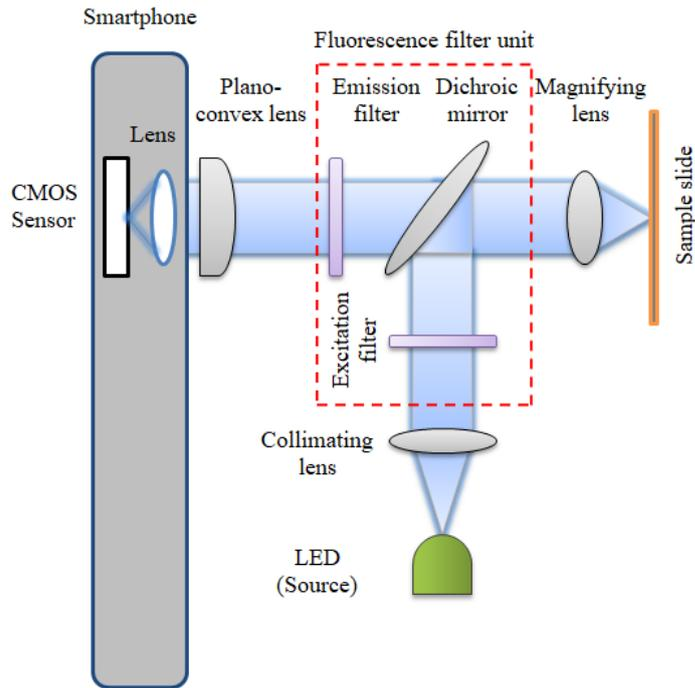
Figure 1: Schematic of the proposed smartphone fluorescence microscope.
