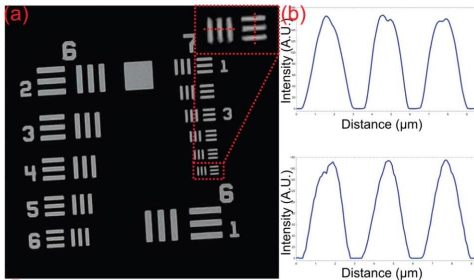
Fig.3 (a) Image of a USAF-1951 resolution test target acquired under BF illumination showing spatial resolution of the microscopic system up to Group 7 Element 6 ( $2.19 \mu\text{m}$ ); (b) represents the intensity profile of the horizontal and vertical element bars of Group 7 indicated in the dotted red line in (a)
